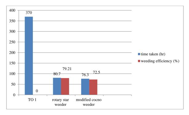
The trail revealed that both the weeders selected for the trails that is rotary and modified cono wedeers has its own strength and limitations. Modified cono weeder can be recommended in the later stages of
